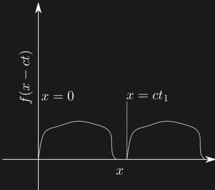
$c$  is the speed of propagation, also known as “phase speed”
